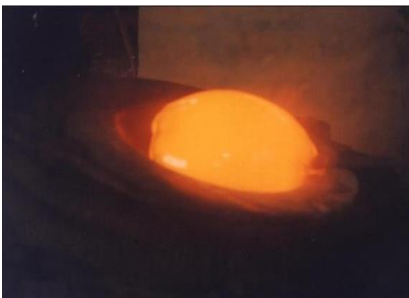
Fig.17. Cooling of the glass mass inside a water basin –
